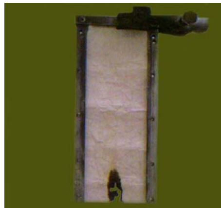
Fig. 1 Mostashari's Flammability Tester with a partly burned fabric at the end of the failure of combustion
